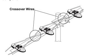
3. Set up the mast, then rotate it so the antenna's shorter elements point toward the broadcast antennas of the stations you want to receive.
